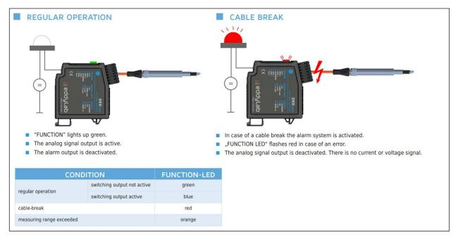
The following figure illustrates the function of the cable break monitoring:
